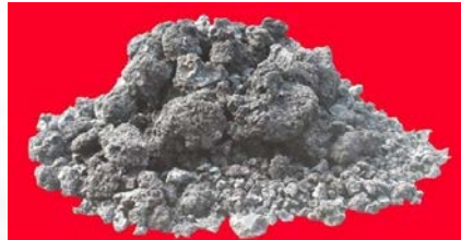
Anode mud: gold, silver, selenium, tellurium
