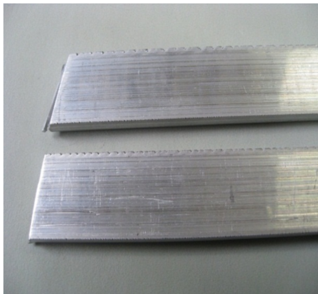
图6 挤制合金扁排边部裂纹 ( V=4\text{ rpm} , T=410^{\circ}\text{C} )
