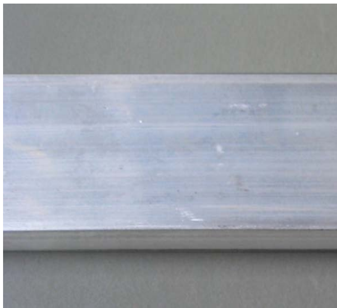
图8 挤制合金扁排 ( V=4.5 rpm, T=447^{\circ}\text{C} )
