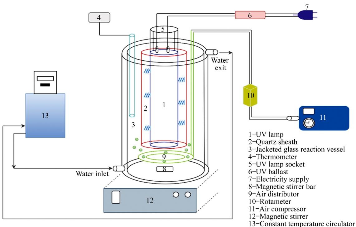
**Figure S4** Schematic representation of the photoreactor system
