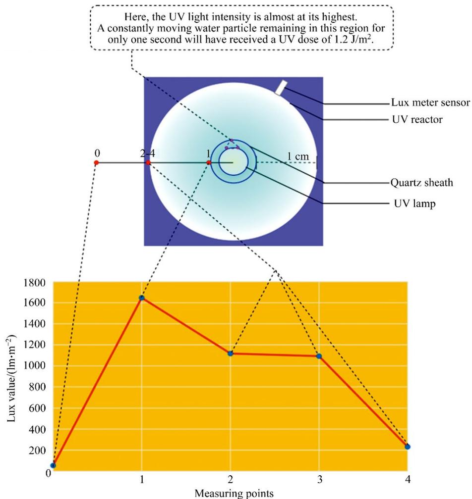
**Figure S6** Beam distribution and lux value measurement results at different points/conditions in a central single UV (185nm-48W) lamp reactor
