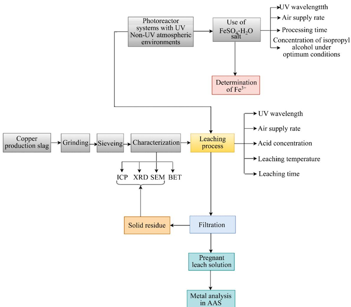
**Figure S3** Proposed experimental flow sheet
