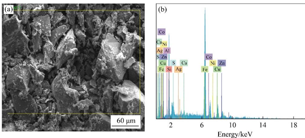
Figure S2 SEM microphotograph and EDX analysis of the copper slags
