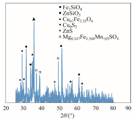
Figure S1 XRD pattern of the copper slags
