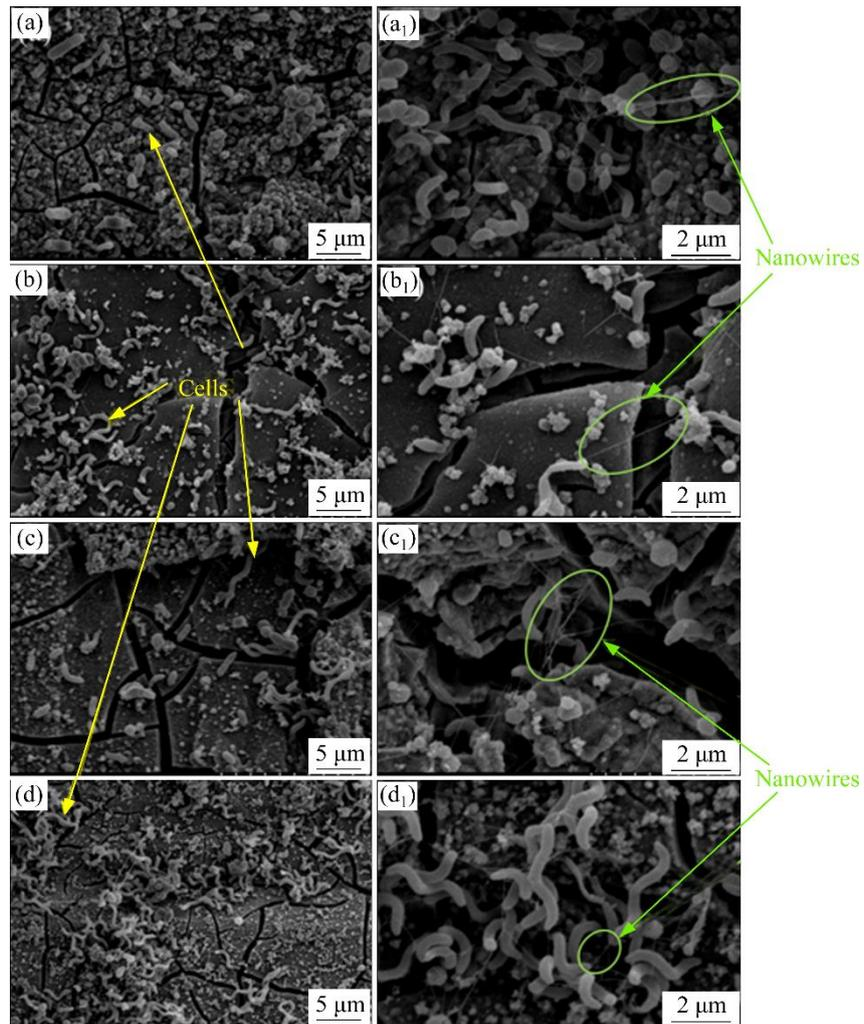
**Figure S1** Surface morphology of AZ31B magnesium alloy coupons after 7-day incubation with carbon source addition of 0% (a, a<sub>1</sub>), 1% (b, b<sub>1</sub>), 10% (c, c<sub>1</sub>) and 100% (d, d<sub>1</sub>)
