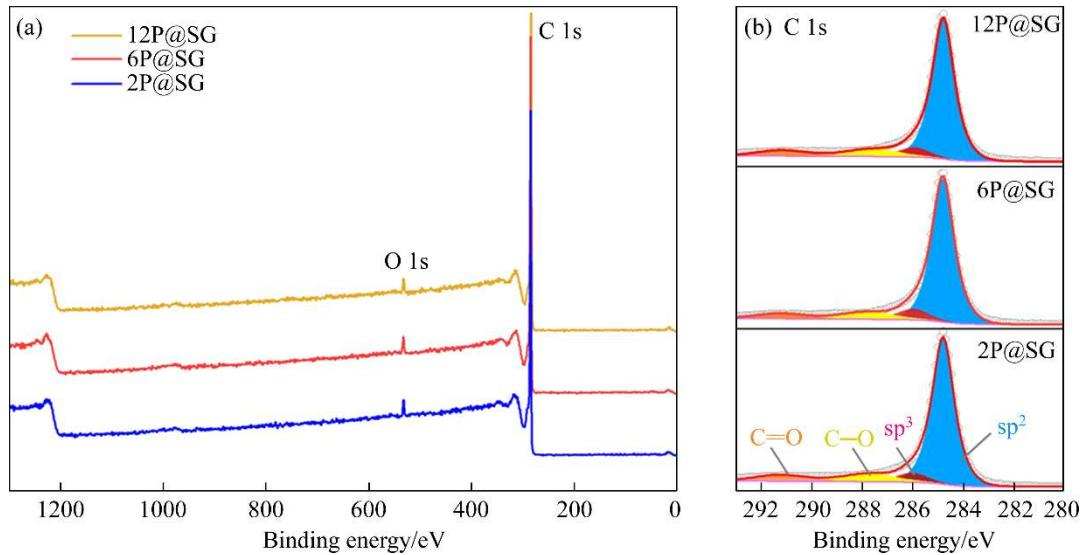
**Figure S4** XPS spectra of 2P@SG, 6P@SG and 12P@SG
